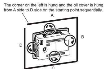
Please confirm all surroundings. Check whether the rubber packing is fitted correctly into the groove on the under side of the GOT front panel, and then whether the protective cover for oil securely covers the rubber packing part to prevent invasion of liquids into the board.
